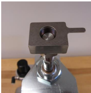
Figure 11: Jaw screwed 1/2-2/3 onto shaft
