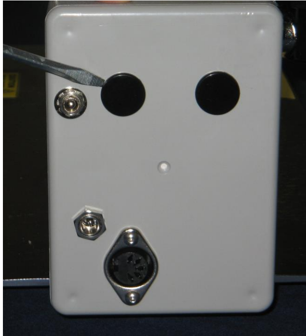
Figure 3: Removing Access Hole Plugs
