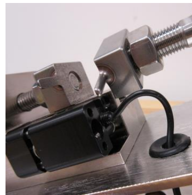
Figure 12: Jaw screwed on too far and slipped off jaw block
