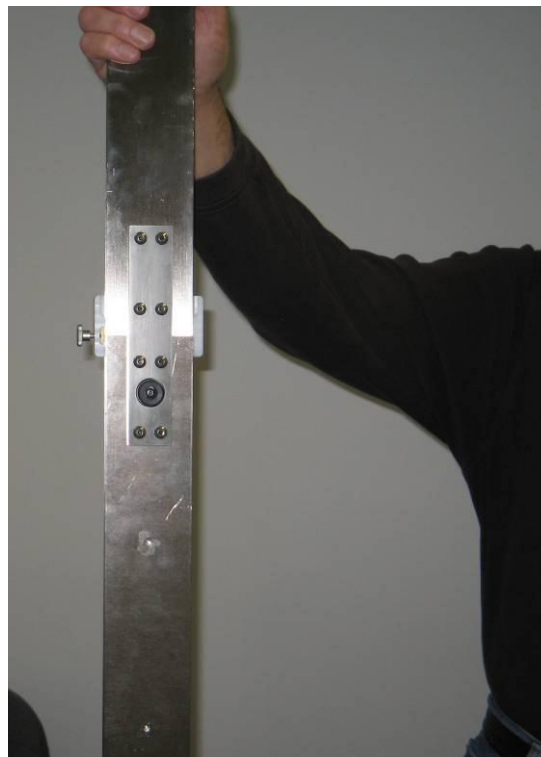
Figure 3: Placing the extension on the base
