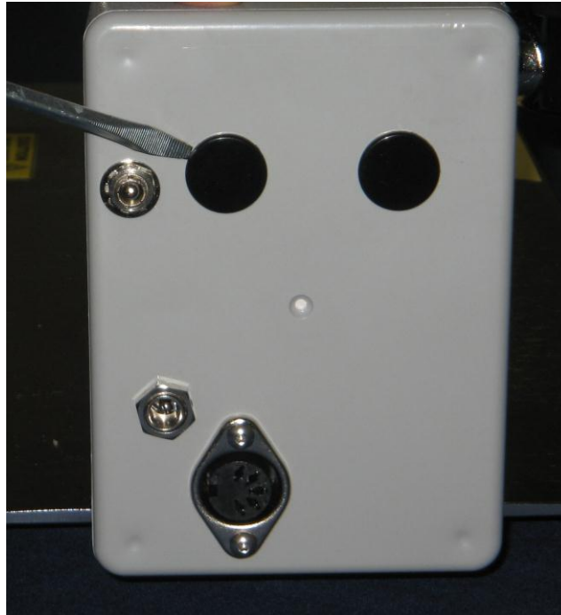
Figure 3: Removing access hole plugs
