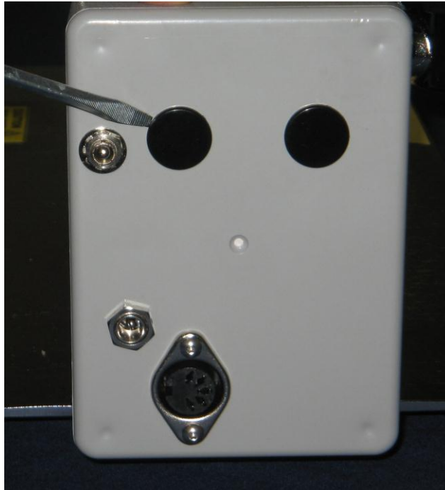
Figure 3: Removing Access Hole Plugs
