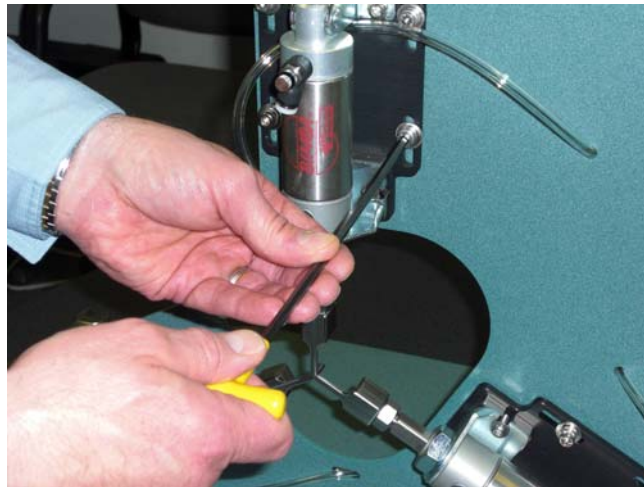
Figure 2: Breaking the cylinder plate loose
