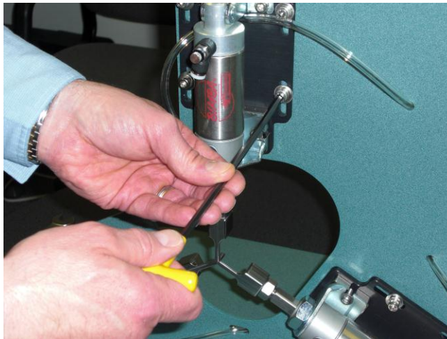
Figure 2: Breaking the cylinder plate loose
